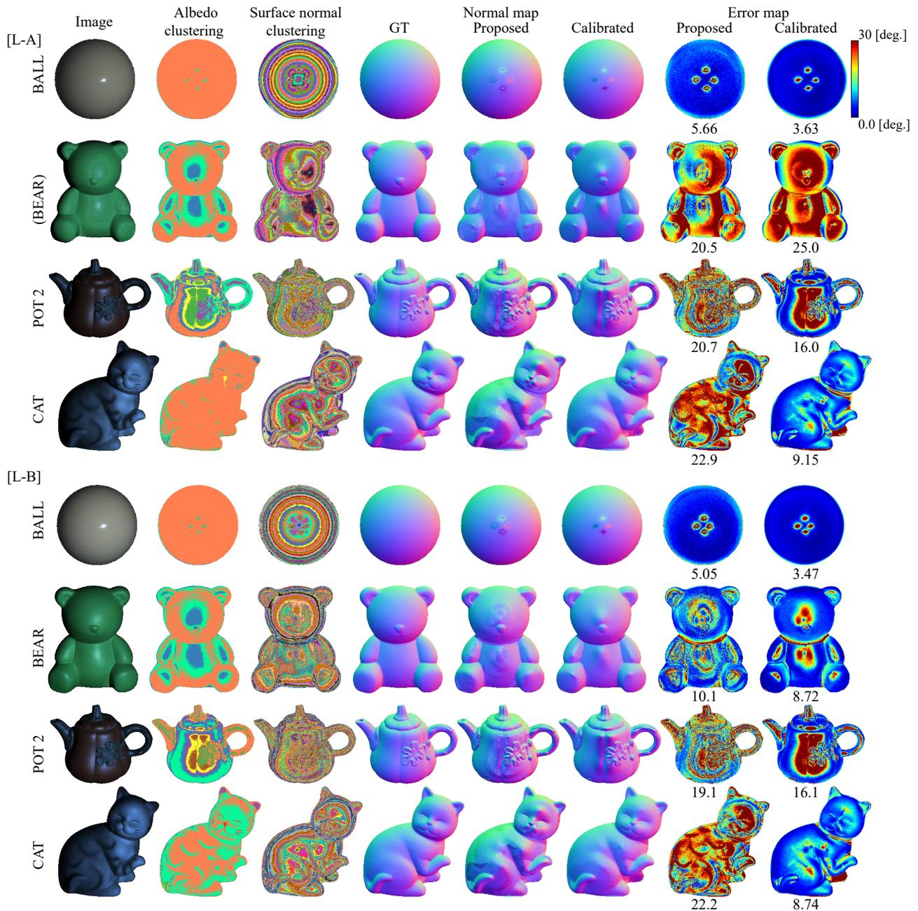
Figure S.5: Estimation results for the DiLiGenT dataset under the two sets of light directions, L-A and L-B. For each row, we show one of the input images, results of albedo and surface normal clustering, the ground-truth and estimated normal maps for each method, and corresponding error maps. For each error map, we show the mean angular errors in degrees. Note that the BEAR scene under L-A contains error, resulting in significant estimation errors for both methods.
