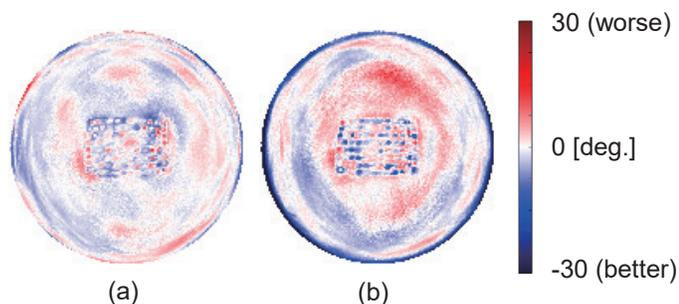
Fig. 14. Comparison of shadowing probability  $p$  on ball scene. (a) and (b) are difference of the error maps of "Proposed" and "Proposed w/o SL" in case  $p = 0.05$  and  $p = 0.9$ , respectively. Pixels whose normal estimation accuracy is improved by the shadow layer are shown in blue, otherwise in red.
