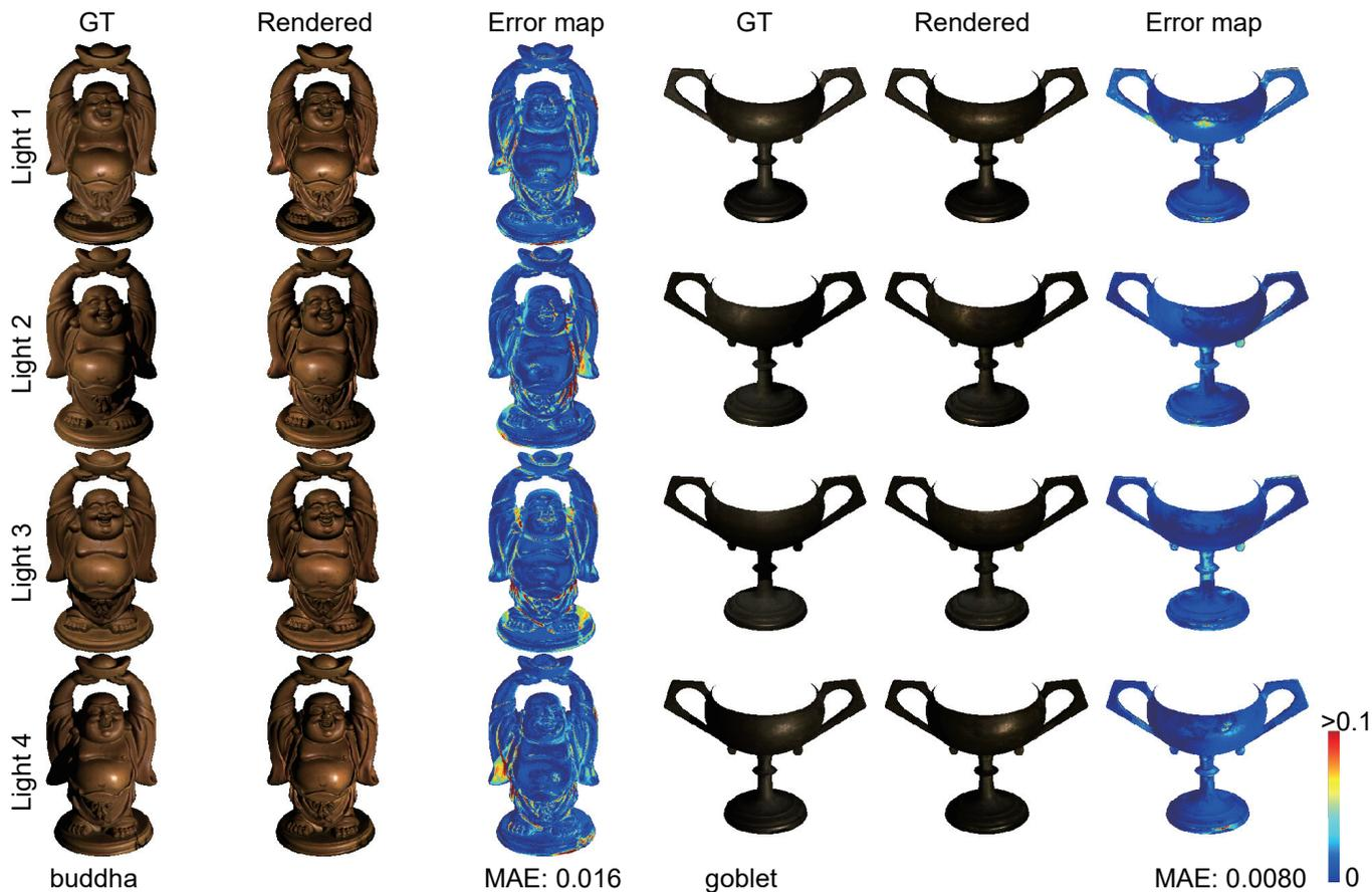
Fig. 9. Rendered results with the estimated BRDFs and the ground truth normal maps for DiLiGenT. *buddha* is the object with non-specular materials and *goblet* is made of metal materials. We apply Gamma correction with  $\gamma = 0.8$  to the ground truth and rendered images for visualization. The light conditions Light 1 to Light 4 are from 96 DiLiGenT light conditions.
