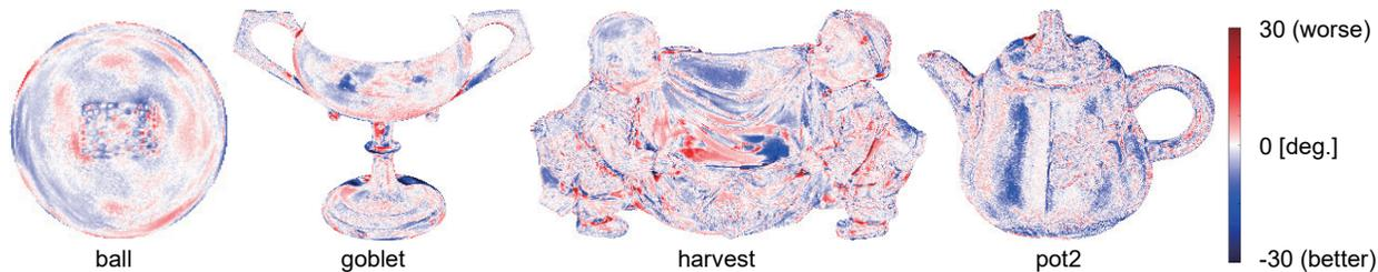
Fig. 12. Improvement by shadow layer. We show a difference map of the error maps of “Proposed w/o SL” and “Proposed”. Pixels whose surface normal estimation accuracy is improved by the shadow layer are colored in blue, otherwise in red.
