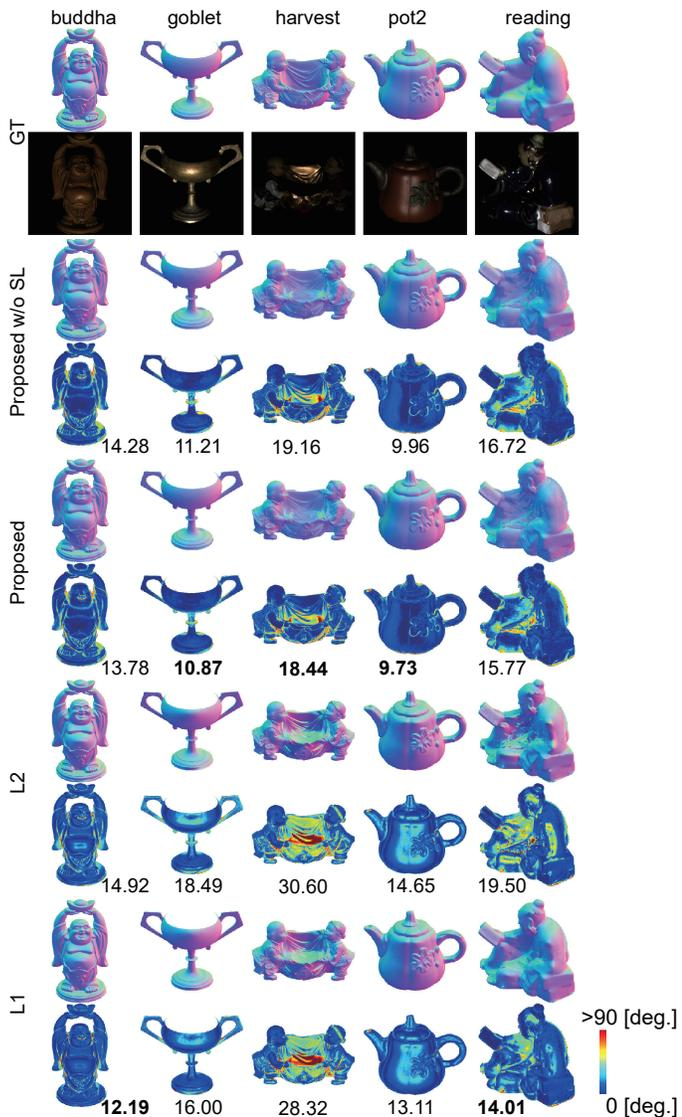
Fig. 8. Surface normal estimation result for real-world scenes from DiLiGenT [51]. In each row, a normal map is shown on top of an error map. The numbers represent Mean Angular Error (MAE) in degree. GT means the ground truth, and figures under GT are examples of observed images. The contrast of observation images is adjusted for better visualization.
