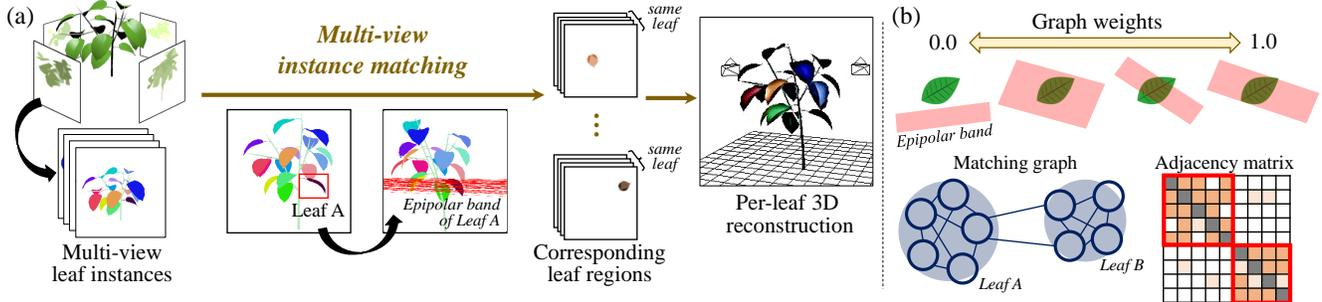
Figure 1: Overview of our method. (a) Proposed pipeline for per-leaf 3D reconstruction. (b) Multi-view instance matching using MRF optimization over a graph where edge weights are defined as the intersection of an epipolar *band* and a leaf instance. After spectral clustering, block diagonals indicate a set of corresponding leaf instances.
